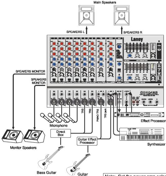
Connect mics or instruments, such as keyboards. to the channel input jacks 1-10.
