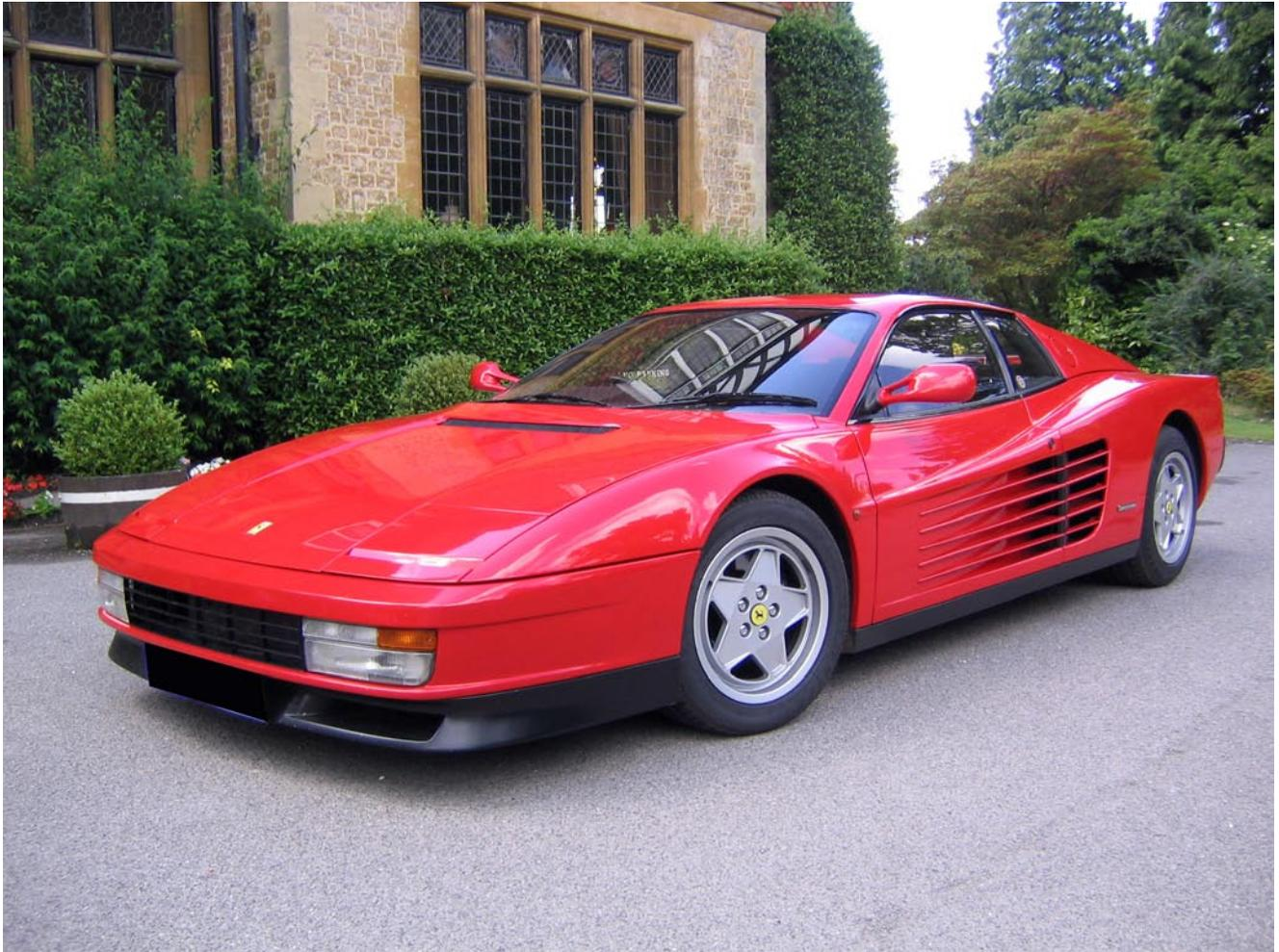
A later model Testarossa is easy to spot. Here is a perfect example as the car has two side mirrors and five bolt wheels.
