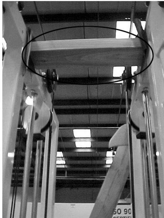
Figure 1. SM22 on pallet (cross bracing circled).
