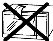
The oven can be operated only if the oven door is firmly closed.
