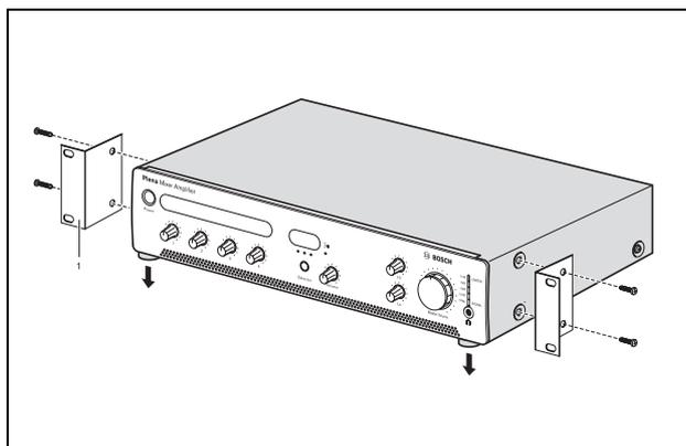
figure 3.1: Installing the unit in a rack
