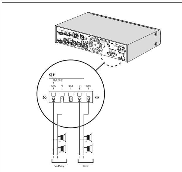
figure 4.9: Connecting speakers
