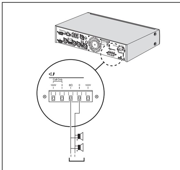
figure 4.10: Connecting speakers
