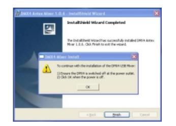
Make sure either the USB cable is unplugged, or power is removed from the DMX-4. Then click "OK".
