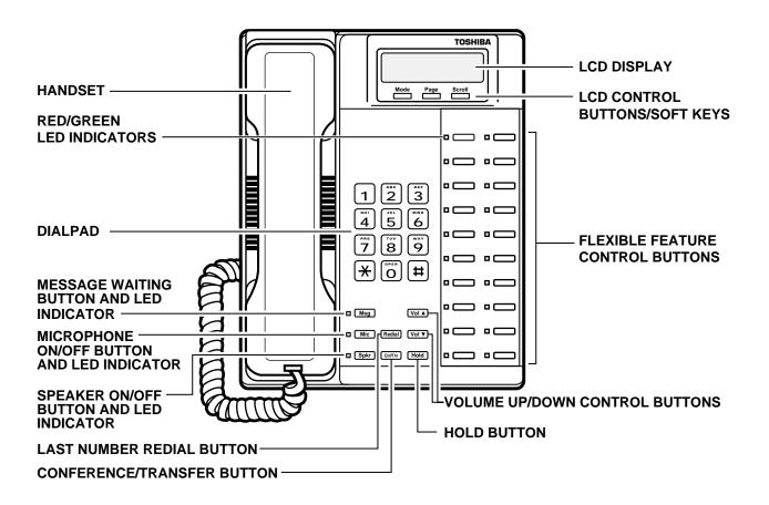
Figure I-2 20-button Digital Speakerphone with Liquid Crystal Display
