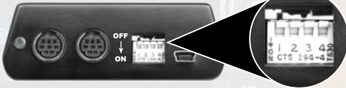
Fig. 1 Side view of interface with dip switches in correct position
