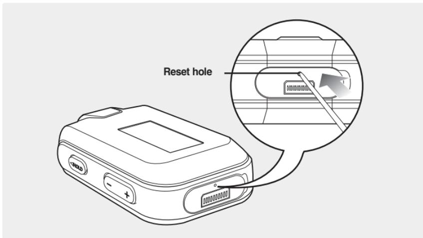
Press the Reset hole at the bottom of the product with a pointed object such as a safety clip.
