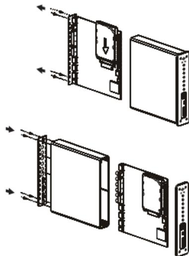
1. Remove four hex screws from the rear (connector panel) using the supplied tool.
