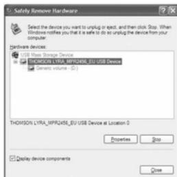
The *Stop a Hardware device* screen appears. Select the device to be stopped again for confirmation and click **OK**.
