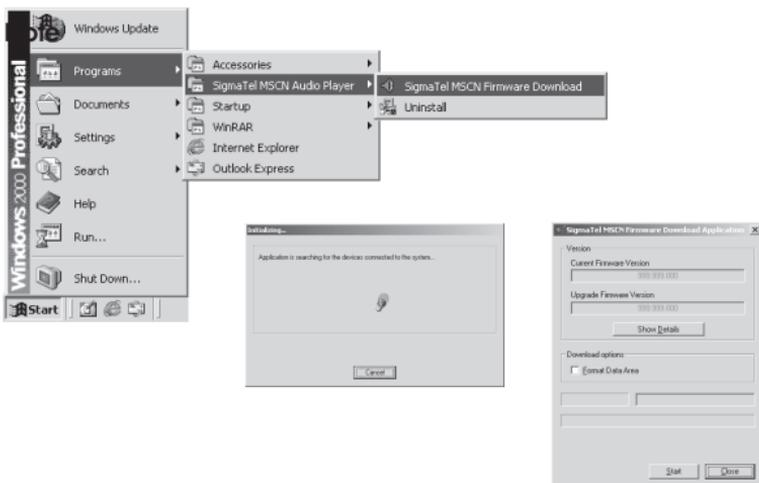
If the flash memory shall be formatted while upgrading firmware *Format Data Area* has to be selected. Click on Yes in the window.
