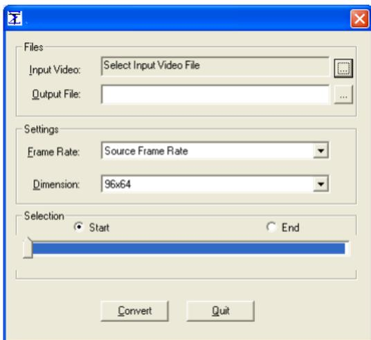
2. Click the button on the right side of **Input Video**, and select the file you want to play. In the window enter the desired **File extension** at **Open**. The unit support .avi / .mpg / .wmv files.
