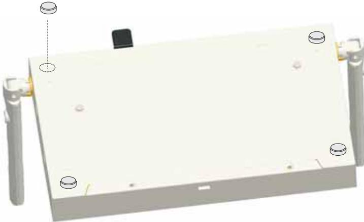
**Mounting on a wall or ceiling** – The access point should be mounted only to a wall or wood surface that is at least 1/2-inch plywood or its equivalent. To mount the access point on a wall or ceiling, always use its mounting bracket. The access point must be mounted with the RJ-45 cable connector oriented upwards to ensure proper operation.
