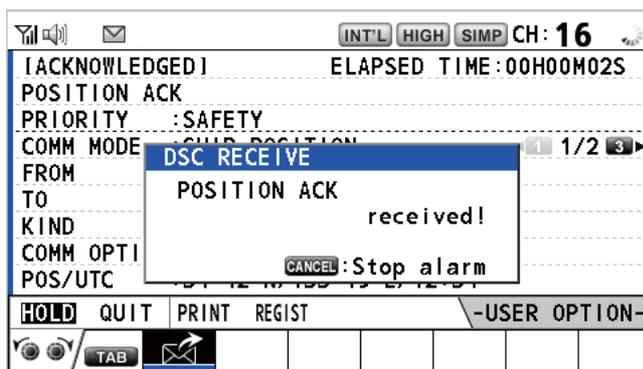
7. Press the **CANCEL** key to silence the audio alarm and erase the pop-up message. There are two types of ACK screens, one with position information and one with no position information.
