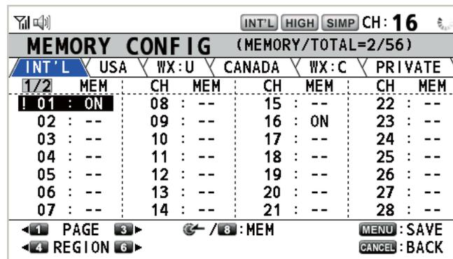
To erase a channel, select a channel to erase then push the **CHANNEL/ENTER** knob or the **8** key. The exclamation mark (!) and [ON] at each side of the selected channel number disappear.
