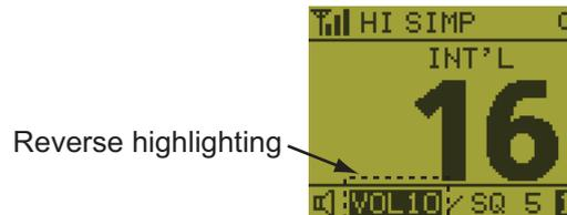
3. Press the **▲** or **▼** key to adjust the volume within three seconds. The time for reverse highlighting is three seconds.
