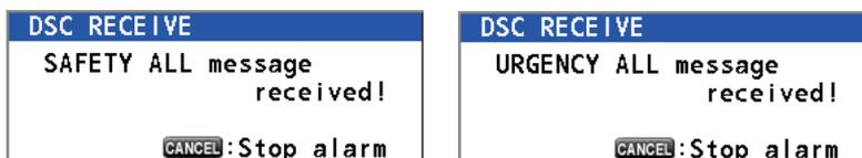
1. Press the **CANCEL** key to silence the audio alarm and erase the pop-up message. The channel is automatically tuned to the received channel.
