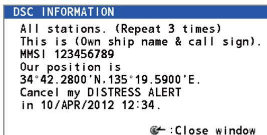
4. Communicate with all ships via radiotelephone referring to the message at step 3.
