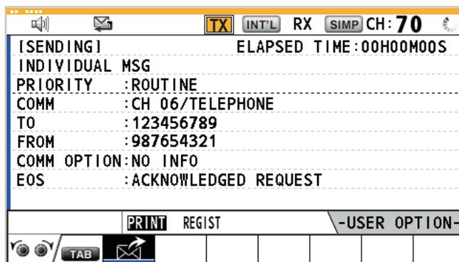
The timer starts counting up the time since the call was sent. After the call is sent, the equipment waits for acknowledgement of the call, showing the WAIT FOR ACK screen as below.
