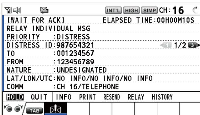
When you receive the distress relay individual acknowledgement from the coast station, the audio alarm sounds and the pop-up message "RELAY INDIVIDUAL ACK received! [CANCEL]: Stop alarm" appears.
