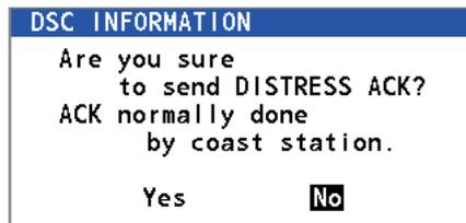
3. If you do not receive the distress acknowledge call from a coast station within five minutes and your ship meets requirements for transmitting the distress acknowledge call, rotate the **CHANNEL/ENTER** knob to select [Yes] then push the knob to send the distress acknowledge call to the ship in distress. The screen changes as below.
