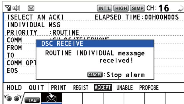
Press the **CANCEL** key to silence the audio alarm and erase the pop-up message. There are three types of ACK transmission; able acknowledge, able to change channel and unable acknowledge. Follow the appropriate procedure below.
