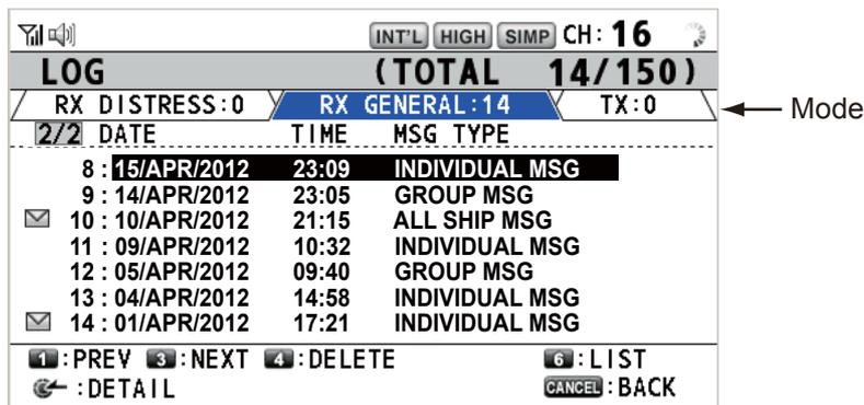
3. Press the **6** key to switch the log file mode in the sequence of [RX DISTRESS] → [RX GENERAL] → [TX] → [RX DISTRESS] → ...
