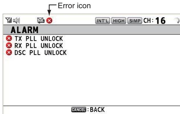
There are three kinds of errors: [TX PLL UNLOCK], [RX PLL UNLOCK], [DSC PLL UNLOCK].
