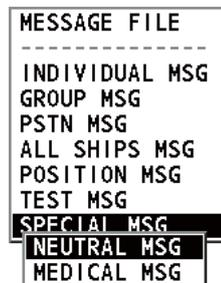
4. Rotate the **CHANNEL/ENTER** knob to select [NEUTRAL MSG] then push the knob. [PRIORITY] is automatically selected to [URGENCY].
