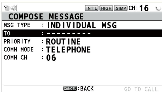
2. Rotate the **CHANNEL/ENTER** knob to select [MSG TYPE] then push the knob.
