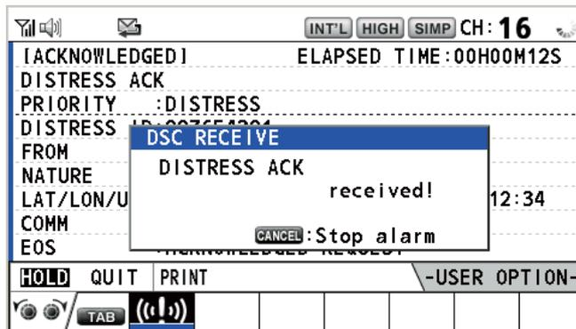
2. Press the **CANCEL** key to silence the audio alarm. Then, the LED stops flashing, and the pop-up message disappears.
