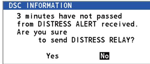
2. Rotate the **CHANNEL/ENTER** knob to select [Yes] then push the knob to open the composing screen for the distress relay individual.
