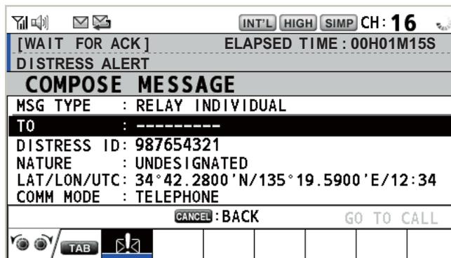
3. Rotate the **CHANNEL/ENTER** knob to select [MSG TYPE] then push the knob.
