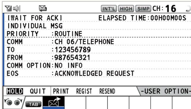
When the ACK is received, the audio alarm sounds and the pop-up message "ROUTINE (or SAFETY, URGENCY) INDIVIDUAL ACK received! [CANCEL]: Stop alarm" appears on the screen as below. The timer starts counting up the time since the ACK was received.
