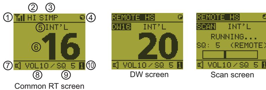
When no terminal has operation right and a remote handset is off hook, the following screen appears.
