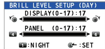
2. To adjust the [DISPLAY] brilliance, rotate the **CHANNEL/ENTER** knob or press the **BRILL** key. (Default setting: 17 for [DAY], 7 for [NIGHT])
