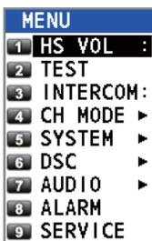
2. Rotate the **CHANNEL/ENTER** knob to select [INTERCOM] then push the knob.
