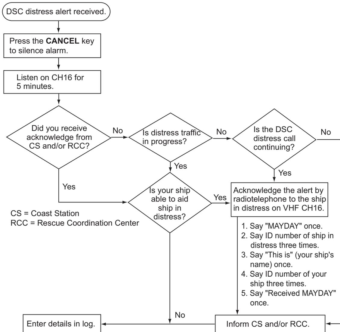
**How to transmit a distress acknowledge call over CH16**
