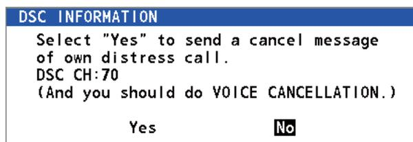
2. Rotate the **CHANNEL/ENTER** knob to select [Yes] then push the knob to send the distress cancel call on CH70. After transmitting the distress cancel call, the following message appears on the screen.
