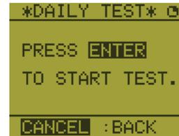
3. Press the **ENTER** key to start the test. You can confirm the test results for FM-8900S with the **1** or **3** key.
