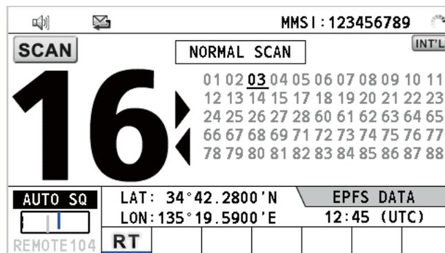
When the receiver detects a carrier and the squelch opens, the scanning is stopped on that channel.
