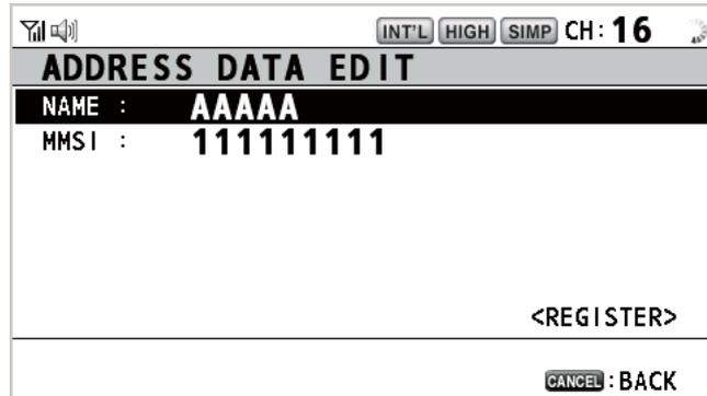
3. Rotate the **CHANNEL/ENTER** knob to select [NAME] or [MMSI] as appropriate then push the knob.
