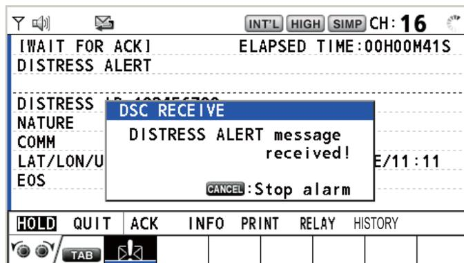
Press the **CANCEL** key to silence the audio alarm. Wait for the distress acknowledge call from a coast station. If you do not receive the distress acknowledge call from a coast station, which usually takes about five minutes from the time of receiving a distress alert, follow the flow charts in this section to determine your action.
