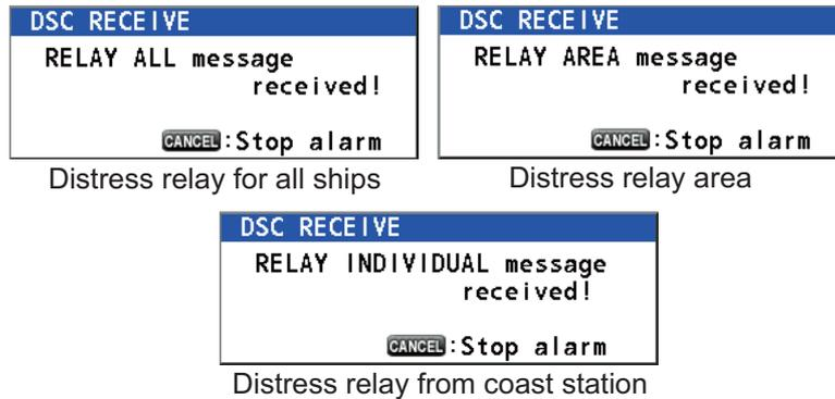
1. Press the **CANCEL** key to silence the audio alarm, stop the flashing of the LED and erase the pop-up message.
