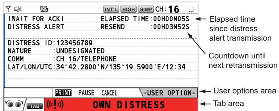
**Note:** If you do not receive the distress alert acknowledge call, the equipment automatically re-transmits the distress alert after 3 min 30 seconds to 4 min 30 seconds. The equipment then awaits the distress alert acknowledge call. This is repeated until the distress alert is acknowledged.
