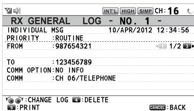
5. Press the **1** key for the previous page and the **3** key for the next page. Rotate the **CHANNEL/ENTER** knob to change the log file (clockwise rotation: to the next log file, counterclockwise rotation: to the previous log file).
