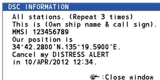
4. Communicate with all ships via radiotelephone referring to the message shown at step 3.
