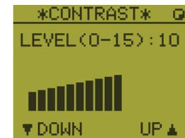
**Note:** The [CONTRAST] setting window automatically closes when there is no menu operation for three seconds.
