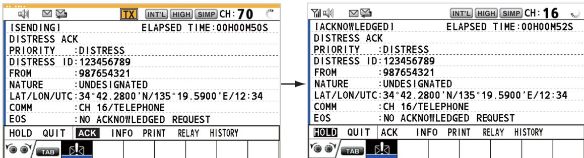
Begin search and rescue operations for the ship in distress, communicating with the ship over CH16 (automatically set). Relay distress alert to a coast station by DSC following the instruction in the next section. Finally, follow the instructions of the coast station.
