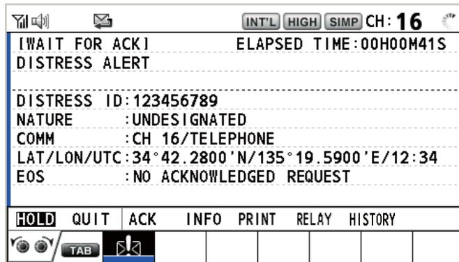
2. Rotate the **CHANNEL/ENTER** knob to select [ACK] in the user options area then push the knob. The following message appears on the screen.
