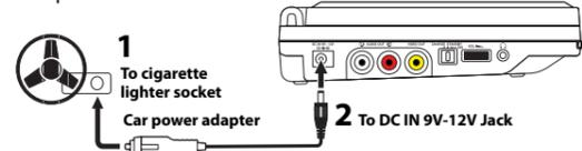
**Warning:** Disconnect the car power adapter when not in use. Not for use in 24V vehicles.
