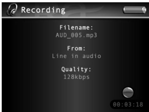
8. Press SELECT to begin recording. Once recording begins, the record screen appears with status and elapsed time, recording quality, and the file name shown.
