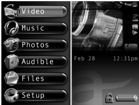
From the main menu, press the up or down arrow button to highlight *Setup*. Press SELECT to view the Setup menu. The following options appear:
