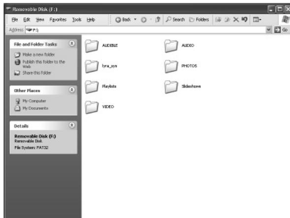
You can copy files to / delete files from the device through Windows Explorer, but you cannot open or edit the files directly from the device. If you want to edit the files, you will need to copy the files from the device to another location (drive) in the system.
