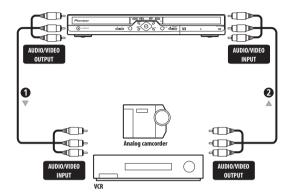
1 Connect a set of audio and video inputs of your VCR or camcorder to a set of outputs on this
