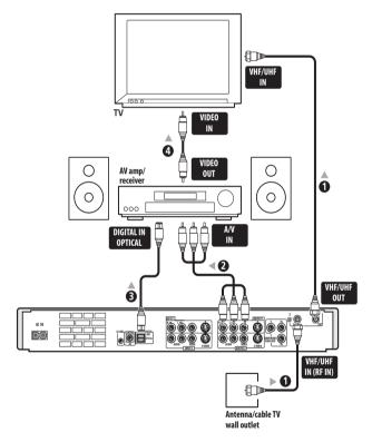
1 Connect RF antenna cables as shown.
