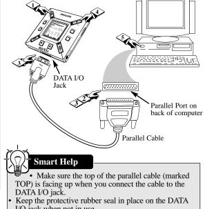
Keep the protective rubber seal in place on the DATA I/O jack when not in use.
