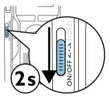
2 To power off, pull down the power switch on the side of the device again and hold for about two seconds.
