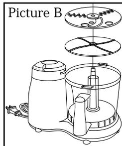
3. Place the Slicing/Shredding Disc on the Drive Shaft. (See Above Picture B)
