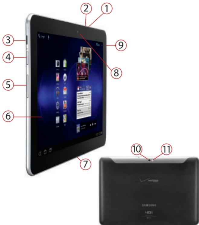
1. **SIM Card Slot:** Install the 4G LTE SIM card, for 4G LTE service.
