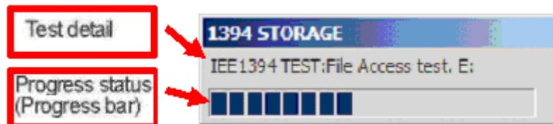
▼ Test detail: The drive under test execution is displayed..
