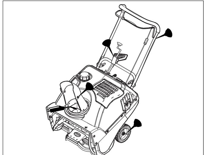
Figure 10. Lubrication points
