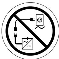
Do not connect an extension cord to the AC/DC converter or the battery charger.
