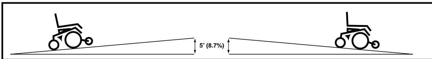
Figure 1. Maximum Safe Angle (Ascending and Descending)
