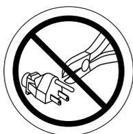
Removal of grounding prong can create electrical hazard. If necessary, properly install an approved 3-pronged adapter to an electrical outlet having 2-pronged plug access.
