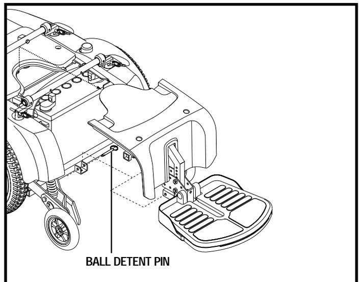
Figure 26. Foot Frame Removal
