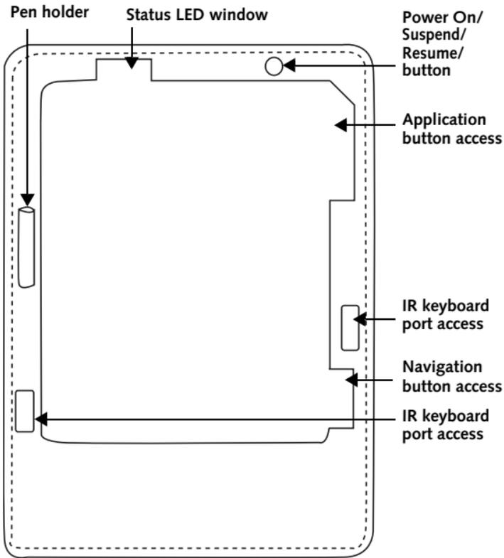
Figure 1. Tablet PC HEC - Front
