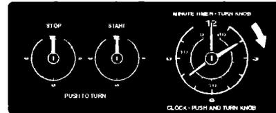
2. Let the Minute Timer Knob pop out. Turn clockwise until Minute Timer hand points to OFF. The clock setting will change if you push in the knob when turning.
