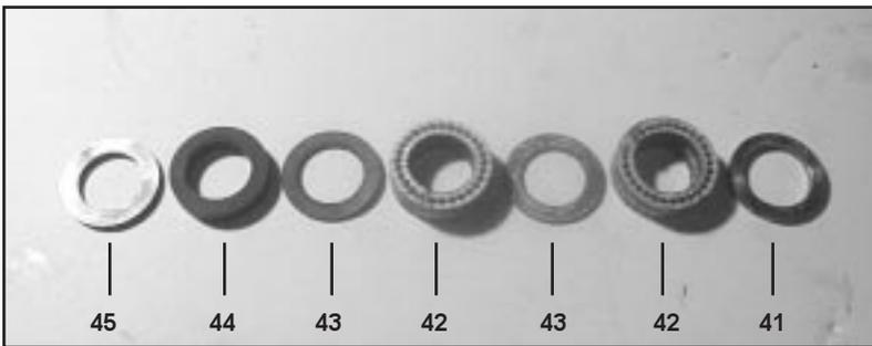
16) Remove support disc (41) seal unit (42, 43, 44) and pressure ring (45) of seal sleeve (38). Examine seals for signs of wear or cavitation, and if necessary, replace.
