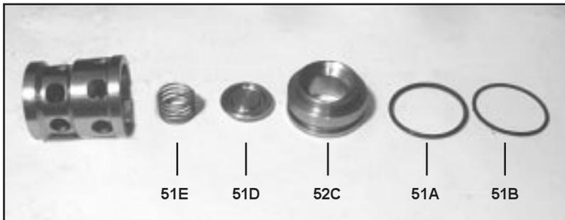
6) Check surfaces of valve plate (51D), valve seat (51C or 52C), o-rings (51A), and support rings (51B). Replace worn parts.
