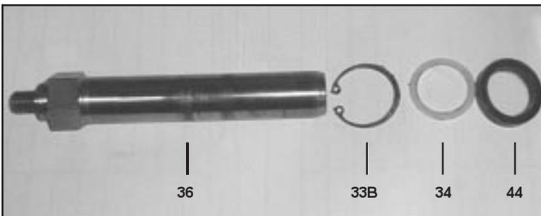
17) Examine plunger (36) for signs of wear or cavitation. If the surface of the plunger is worn, screw out the plunger with a 27mm tool. Clean centering and front surface of crosshead with plunger (25). Thread new plunger carefully through oiled seals in seal sleeve. Coat thread of new plunger lightly with bonding agent (e.g., loctite).
