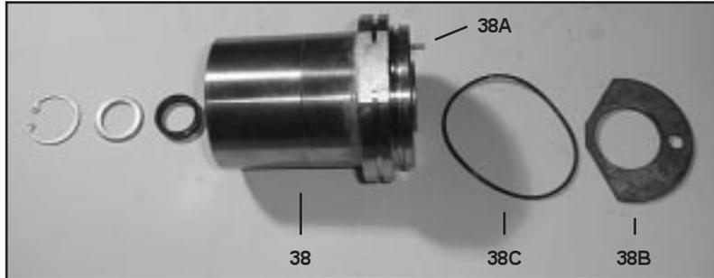
14) Remove circlip ring (48) from seal sleeve (38). Remove spacer disc (47) and seal ring (46) from seal sleeve. Replace worn or damaged parts.
