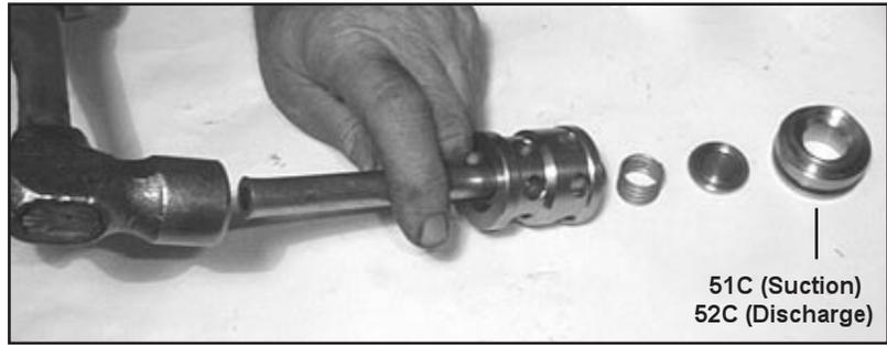
5) Valve seats (51C and 52C) are pressed out of spacer pipe (51F) by hitting the valve plate (51D) with a socket extension.
