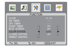
**Note:** The color system item is adjustable only in **AV1**, **AV2** and **SVIDEO** mode. In normal circumstances, please set the color system to **AUTO**, and the set can automatically select the proper color system. If the color is still abnormal, then select the proper color system manually.
