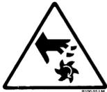
**Never reach into the mix section of the blender without disconnecting the power or air supply. Serious injury can result from getting your hand caught in the rotating mixer!**
