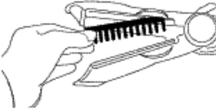
3. There are 2 Straightening Combs included with your hair Straightener. They may be used in any position that works best for you. When inserting both Combs into either the top or the bottom of the unit, be sure the teeth are facing up and the flat side (non-wavy) is against the Straightening Plates. Push down firmly until both Combs are in place.
