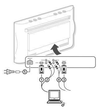
In case of a Multimedia computer, also connect the audio cables to AUDIO OUT R and L ② next to the VGA OUT connector and to the audio inputs of the second VGA monitor.
