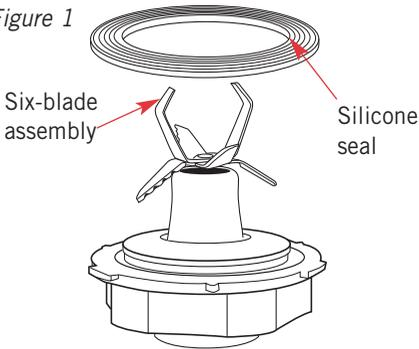
2. Place the six-blade assembly into the glass jug and turn clockwise to secure firmly into position (see Figure 2).
