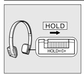
This function stops the unit from responding when a button is pressed.
