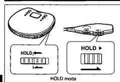
This function causes the unit to ignore short, accidental button presses. (The disc lid can still be opened and closed."
