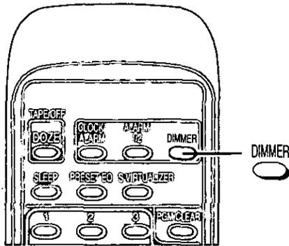
**A Dimming the Display Panel****Remote control only**
