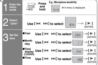
The clock has a monthly accuracy of  $\pm -60$  seconds at room temperature. When replacing the batteries, the clock stops and restarts when you reinsert them and close the battery cover
