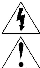
This symbol warns the user that uninsulated voltage within the unit may have sufficient magnitude to cause electric shock. Therefore, it is dangerous to make any kind of contact with any inside part of this unit.
