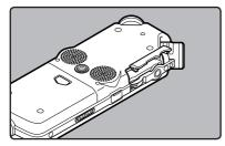
Face the card the correct way and insert it into the card slot as shown in the diagram.
