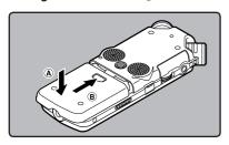
A Slide the **POWER/HOLD** switch in the direction indicated by the arrow, and turn the power on.
