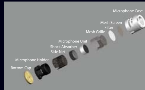
Low-vibration microphone structure
