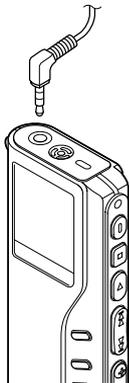
**You can listen to audio playback through the earphone connected to the jack on the recorder or the EAR jack on the remote controller.**
