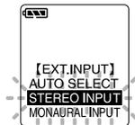
When set to STEREO INPUT, the recorder starts recording in SHQ mode. When set to MONAURAL INPUT, it starts recording in the specified recording mode.
