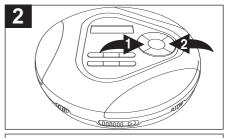
Select a track to be programmed using the Skip/TUNING ₩ ① or № ② button. If using a MP3 disc, see note below.
