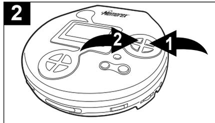
**2** Press the PLAY/PAUSE (▶||)/POWER ON button ⏻ to begin playback. The unit will play all the tracks in random order. When all the tracks have been played, the unit will stop. Press the STOP (■)/POWER OFF button ⏻ to stop Random playback.
