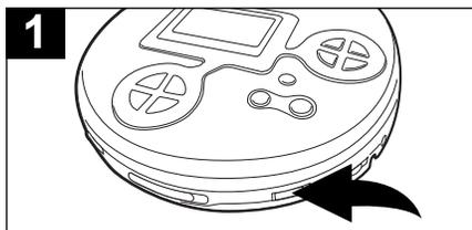
**1** To emphasize the bass, slide the DBBS switch to the ON position. For normal bass, slide the DBBS switch to the OFF position.
