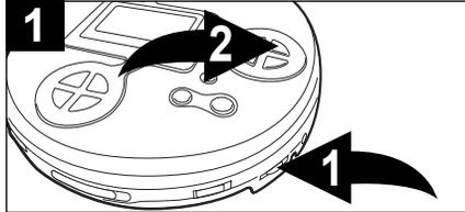
Set the VOLUME control ❶ to minimum and plug the headphone into the PHONES jack. Press the PLAY/PAUSE (▶||) /POWER ON button ❷ to turn the unit on.
