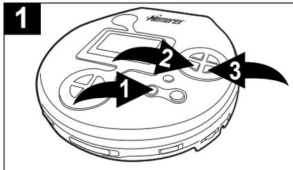
To repeat all files in a directory (MP3 CD only), while in the Stop mode, press the MODE/◀ button ❶ three times; "REP D" will appear in the display. Press the Skip/TUNING DN (◀◀) ❷ or UP (▶▶) ❸ button to select the specific directory that you wish to repeat.
