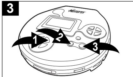
3 Press the ENTER/CLEAR button ❶ and a list of files starting with the selected letter will appear. Press the MODE/◀ ❷ and/or RESUME/▶ ❸ buttons to scroll through the list.
