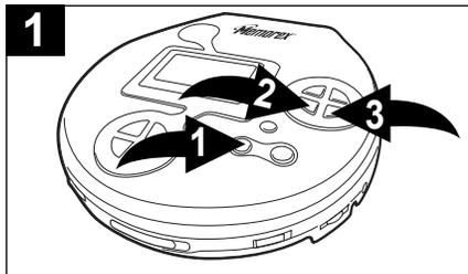
To repeat a single track, while in the Stop mode, press the MODE/◀ button **1** once; "REP 1" will appear in the display. Press the Skip/TUNING DN **2** or UP **3** button to select the specific track that you wish to repeat.
