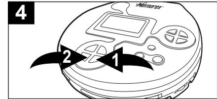
**4** To receive a preset station, simply press the PRESET ▲ ❶ or ▼ ❷ button to select the desired preset.
