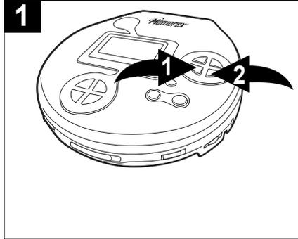
During playback, depress and hold either the Skip/TUNING DN **1** or UP **2** button to move the player forward or backward within a track to locate a specific musical passage. The player will move forward or backward at high speed as long as the buttons are depressed. When you release the Skip/TUNING DN **1** or UP **2** button, normal playback will resume.
