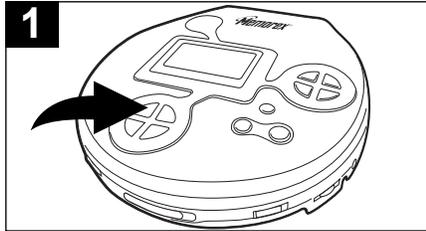
**1** Tune a desired station as described in the previous section. Press the PROGRAM button; the preset number will blink.
