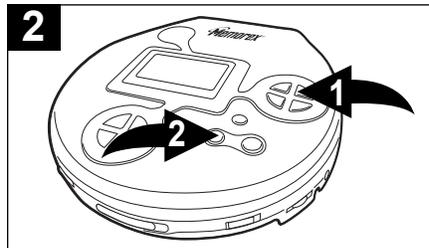
When the desired track number appears in the display, press the PLAY/PAUSE (▶||) /POWER ON button **1** to begin playback. The specific track you selected will be repeated continuously. To cancel Repeat playback, press the MODE/◀ button **2** repeatedly until the mode indicator disappears.
