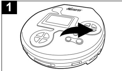
During playback, press and release the Skip/TUNING UP button once to advance the player to the beginning of the next track. Press the Skip/TUNING UP button repeatedly to advance the player to higher numbered tracks.
