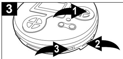
3 Press the PLAY/PAUSE (▶||) /POWER ON button ❶ to begin playback; the current track and elapsed playing time (CD information and folder will also appear, if using MP3) will blink in the display. Adjust the VOLUME control ❷ and DBBS switch ❸ as desired.
