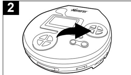
During playback, press and release the Skip/TUNING DN button once to move the player back to the beginning of the currently playing track. Press the Skip/TUNING DN button repeatedly to move the player back to lower numbered tracks.
