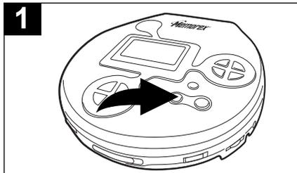
**1** While in the Stop mode, press the MODE/◀ button four times (five times if an MP3 CD with multiple directories is inserted); "RANDOM" will appear in the display.
