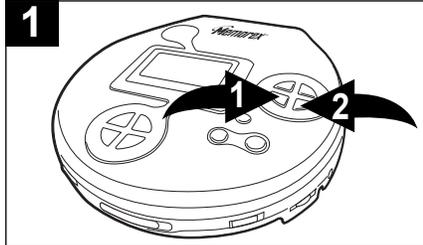
After you insert the disc into the CD player and the total number of tracks and time appear on the display, you may press either the Skip/TUNING DN or UP button to select a specific track for playback.
