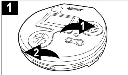
1 Press the PLAY/PAUSE (▶||) /POWER ON button ❶ to turn the unit on. Slide the FUNCTION switch ❷ to the CD position.
