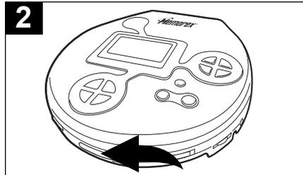
2 Slide the CD Door OPEN switch to the right to open the CD compartment. Gently press a disc, label side up, onto the spindle until it locks in place. Close the CD compartment lid; the total tracks (and folders, if using MP3) will appear in the display. "Door Open" will appear in the display when the CD Door is opened.
