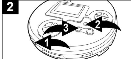
Slide the FUNCTION switch ❶ to the RADIO position. Press the MENU/ESP/BAND button ❷ to select a band (AM or FM). If listening to FM, press the MODE/◀ button ❸ to select Stereo or Mono.
