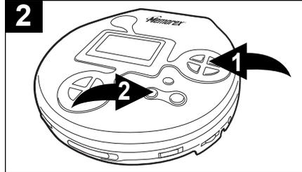
Press the PLAY/PAUSE (▶||)/POWER ON button ❶ to begin playback. All tracks on the disc will be repeated continuously. To stop Repeat playback, press the MODE/◀ button ❷ repeatedly until the mode indicator disappears.
