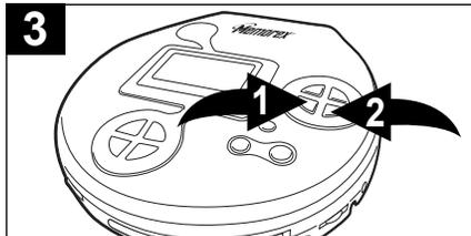
Press and release the Skip/TUNING DN ◀◀ ❶ or UP ▶▶ ❷ button to tune a station. Press and hold the Skip/TUNING DN ◀◀ ❶ or UP ▶▶ ❷ button for Auto Scan tuning (see below).
