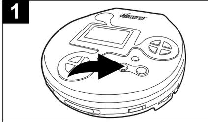
**1** While in the Stop mode, press the MODE/◀ button three times (four times if an MP3 CD with multiple directories is inserted); "INTRO" will appear in the display.
