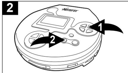
Press the PLAY/PAUSE (▶||)/POWER ON button ❶ to begin playback. All files in the selected directory will be repeated continuously. To stop Repeat playback, press the MODE/◀ button ❷ repeatedly until the mode indicator disappears. See page 16 for more info on MP3 format.
