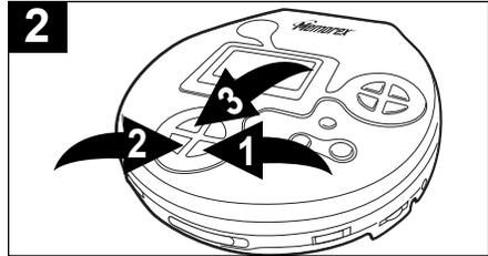
**2** Within ten seconds, select the desired preset using the PRESET ▲ ❶ or ▼ ❷ button to set the memory. Press the PROGRAM ❸ button to confirm.
