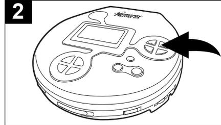
When the desired track number (and file number if using MP3) appears in the display, press the PLAY/PAUSE () /POWER ON button. Playback will begin with the track (or file) you selected.
