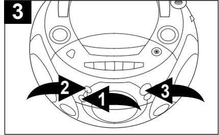
To start from a specific track, locate the track using the **SKIP/Search** ◀◀ ① or ▶▶ ② button and press the **PLAY/PAUSE** (▶/||) button ③.
