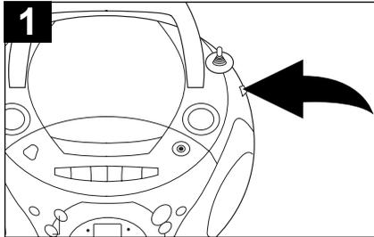
Slide the **FUNCTION** switch to the **TAPE** position.
