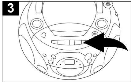
When you are ready to begin recording, press the RECORD (●) button. The PLAY (◀) button will also engage. The tape will begin moving and all of the material from your selected source will be recorded on the tape.
