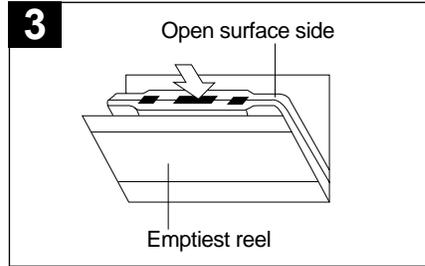
Insert a pre-recorded cassette into the slots in the Cassette Door with the open end facing up and the full reel on the right side. Close the cassette door.
