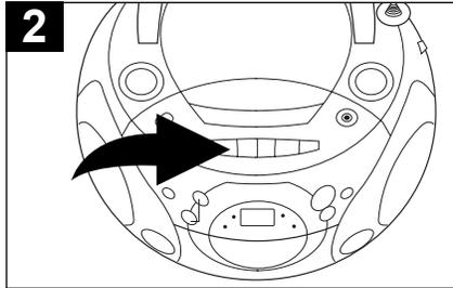
Press the **STOP/EJECT** (■▲) button to open the Cassette Door.
