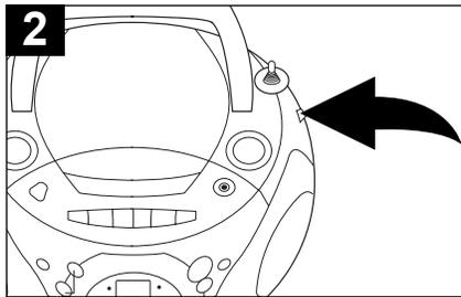
Slide the FUNCTION switch to select the function you wish to record, either AM, FM ST. or CD, and operate that function according to its own instructions.
