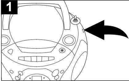
1 Slide the **FUNCTION** switch to the CD position; the **POWER ON** indicator will light. Insert a CD as described in the **TO INSERT A CD** section on page 6.
