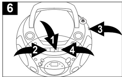
If you wish to listen to your recording immediately, press the cassette REWIND (▶▶) button ❶ until the tape rewinds to the beginning, then press the STOP/EJECT (■▲) button ❷. Slide the FUNCTION switch ⊕ to the TAPE position and press the PLAY (◀) button ❹ to begin playback.
