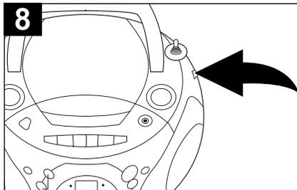
When you have finished listening, slide the **FUNCTION** switch to the **TAPE/POWER OFF** position.
