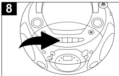
To stop playback before the tape ends, press the **STOP/EJECT** (■▲) button. The **PLAY** (◀) button is released and the tape motor shuts off.
