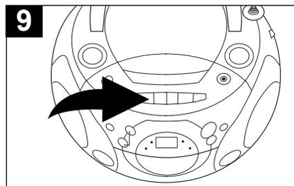
When the tape reaches the end, the auto-stop mechanism activates, the **PLAY** (◀) button is released and the tape motor shuts off. Press the **STOP/EJECT** (■▲) button to open the Cassette Door and remove the tape.
