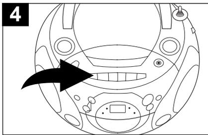
To avoid recording unwanted material, such as radio commercials, use the PAUSE (||) button to stop the recording temporarily. Release the PAUSE (||) button to begin recording again.
