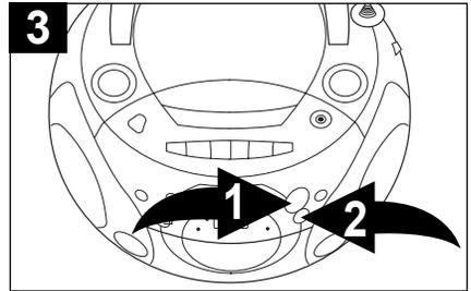
3 Press the **PLAY/PAUSE** (▶/||) button ❶ to begin playback and the unit will play the entire disc over and over until the **STOP** (■) button ❷ is pressed.
