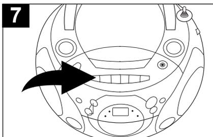
To pause playback momentarily, press the **PAUSE** (||) button. The tape movement stops but the tape motor is still running. Press the **PAUSE** (||) button again to release Pause and resume normal playback.
