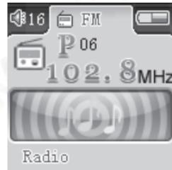
Press [MENU] button to switch among Radio, Scan, Store, Recording and Return under FM menu. The Operations are as the following:
