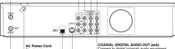
Plug into the power source. Connect to digital (coaxial) audio equipment.
