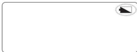
**Always exchange both batteries** to operate the Portable MP3-CD player with full power or connect the player with the mains adapter to the mains socket.
