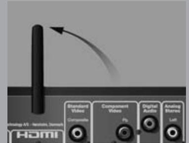
For an optimal wireless transmission, remember to turn the antennas upwards.
