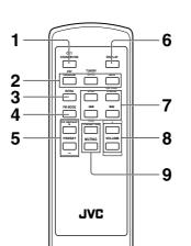
1 STANDBY/ON **U/I** button 2 CD/RANDOM button TUNER/BAND button TAPE button 3 INTRO button 4 FM MODE button 5 PRESET + /CD REPEAT button PRESET - button
