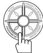
The tuned station in step 1 is stored in the preset number selected in step 3.
