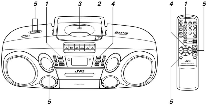
**1 Press the CD/RANDOM button to enter CD mode, if the unit is in TUNER or TAPE mode.**
