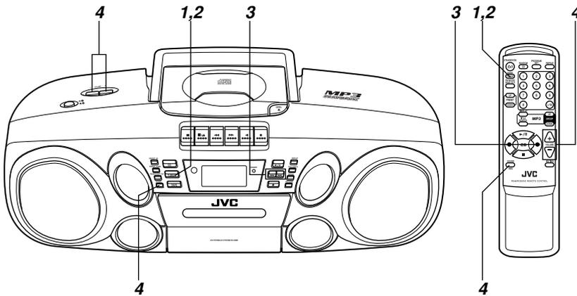
**1** Press the TUNER/BAND button to enter TUNER mode.
