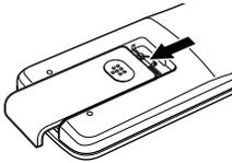
**2** Insert two R03 (UM4)/AAA (24F)-size batteries. Insert the batteries with the  $\oplus$  and  $\ominus$  terminals matching the indication inside the battery compartment. Insert the  $\ominus$  ends first.
